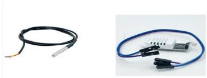
Figure 2: Temperature sensors used in the monitoring system: DHT22 and DS18B20.
