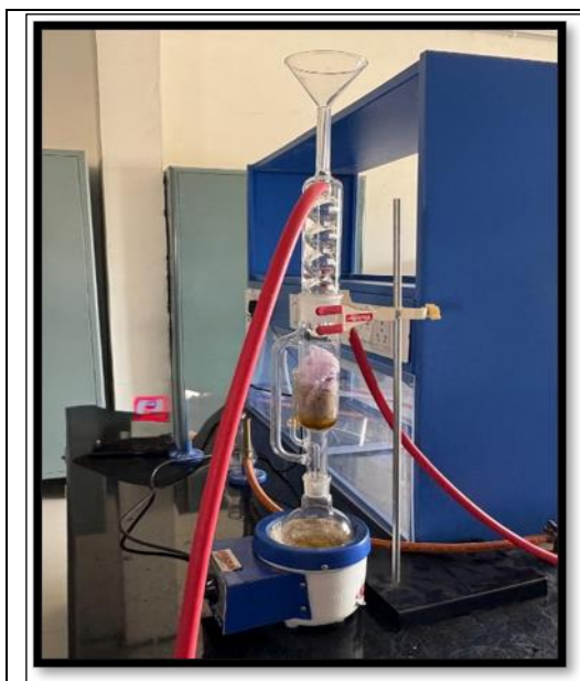
Figure 3: Soxhlet Extraction using Ethanol
