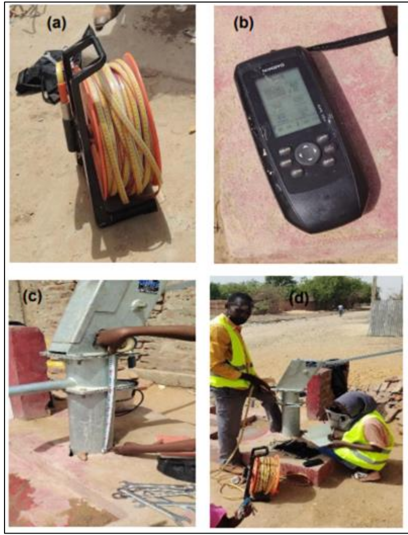
Figure 2: Field studies: (a) piezometric prob; (b) GPS (GARMIN); (c) and (d) water level measurements.
