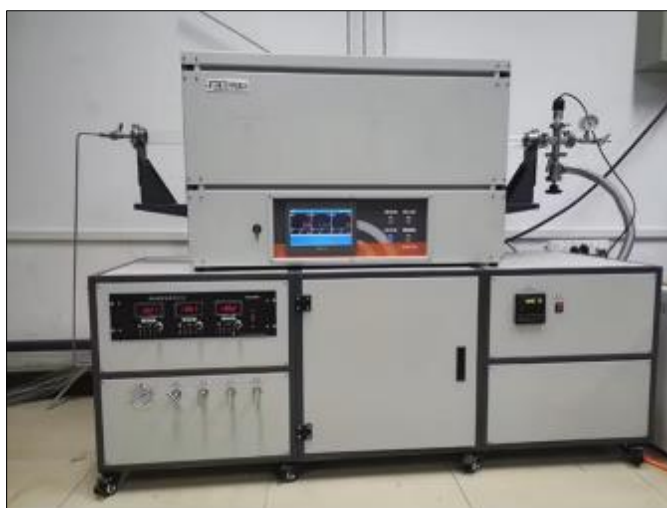
Figure 1 Horizontal tubular furnace used for the pyrolysis of agro-industrial biomass under an inert nitrogen atmosphere for biochar production.2.3. \text{TiO}_2/\text{Fe}_3\text{O}_4 Modification
