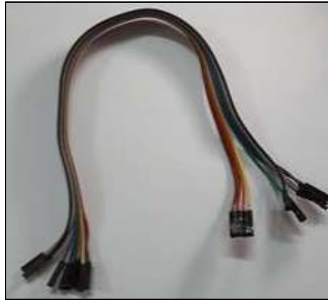
Figure 3 Jumper wires with different standards
