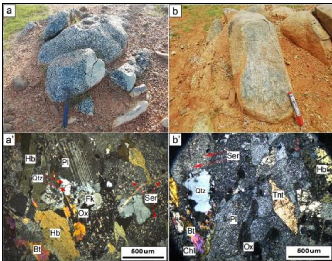
Figure 8 (a and b) Photographs showing (a) porphyritic quartz diorite, (b) quartz microdiorite, and (c and d) Microphotographs showing the mineralogical composition of (c) porphyritic diorite and (d) microdiorite. Pl: plagioclase, Hb: hornblende; Bt: biotite, Qtz: quartz, Fk: K-feldspar, Tnt: titanite, Chl: chlorite and Ox: Fe-Ti oxides
