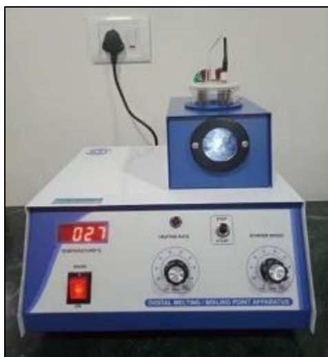
Figure 3 Digital Melting/Boiling Point Apparatus used for determination of melting and boiling points of pharmaceutical compounds and samples
