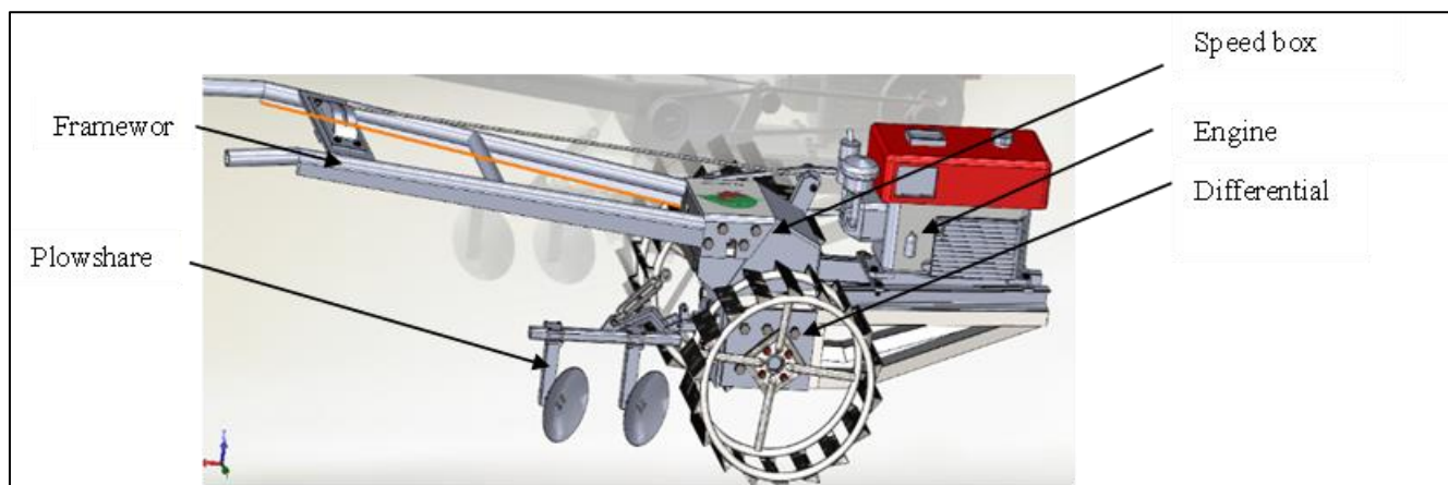
Figure 5 Final assembly in retained solutions of a tiller
