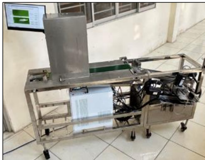
Figure 11 Photograph of the designed vaccination system
