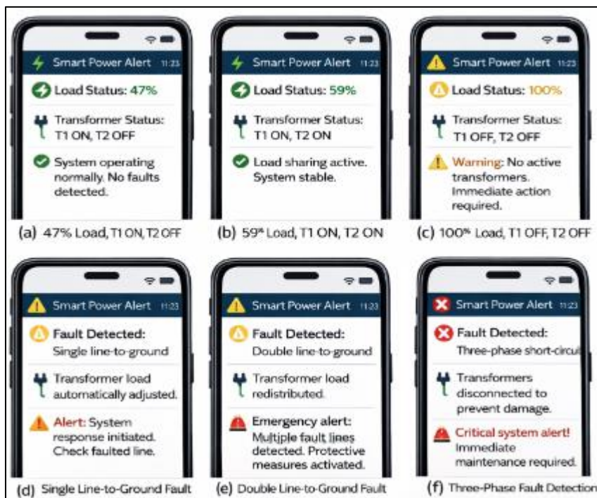
Figure 12 Mobile interface of the proposed system showing real-time load status (47%, 59%, 100%) and detection of SLG, DLG, and three-phase faults with automated transformer control and alert generation
