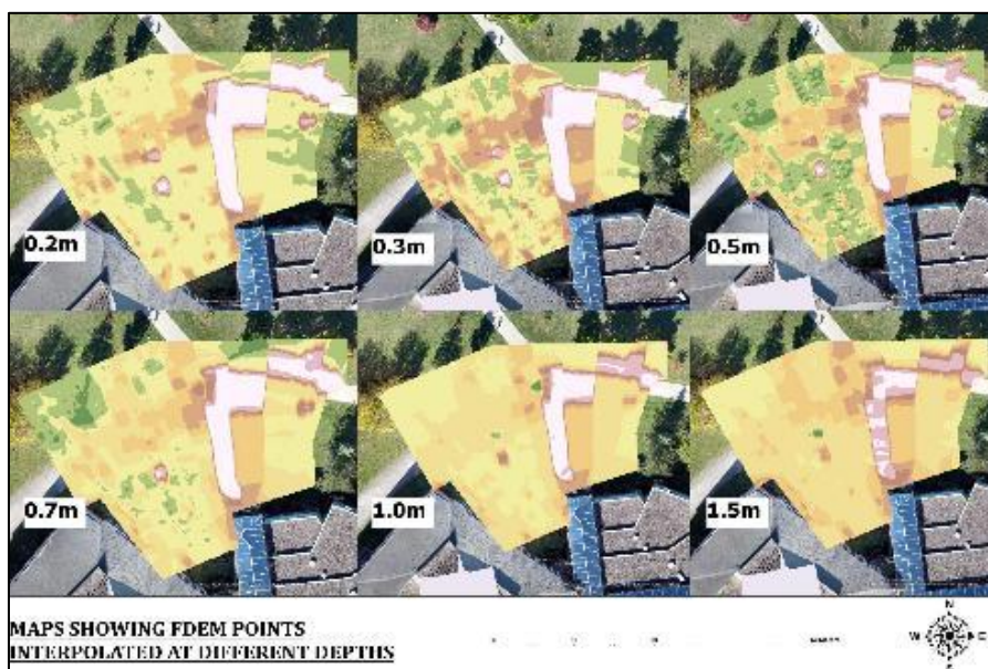
Figure 6 FDEM Interpolated lines created in ArcGIS pro using Kriging operator
