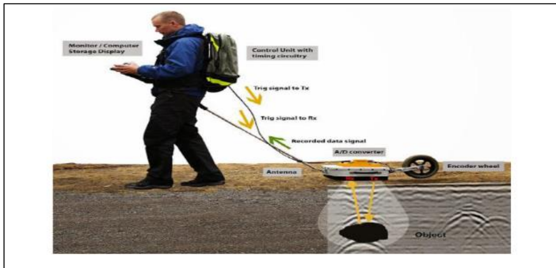
Figure 2 Components of a GPR System
