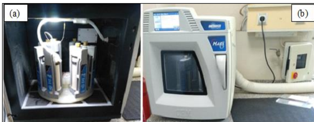
Figure 2 Image of CEM Microwave digestion system. (a) Vessels loading, (b) At the starting of microwave operation (Chapiou, 2022)
