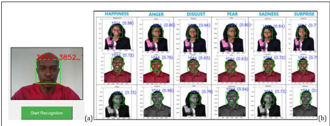
Figure 3 Face recognition output showing detected faces with assigned Unique Identification Numbers (UIDs) (a) Recognized face displaying UID 3852 linked to NIN record (b) Recognized face of the same persons recognized under a different facial expression
