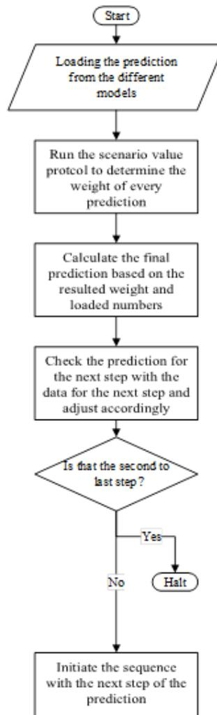
**Figure 6** The scenario evaluator makes a prediction based on the outcome of all the procedures. The prediction would then be compared with the actual numbers from the next step that is stored in the data to determine and improve the prediction accuracy.
