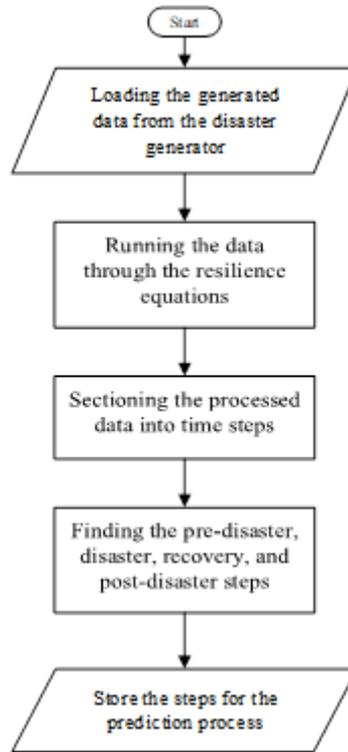
**Figure 1** The raw data coming from the disaster generator gets processed into meaningful data by applying the resistance equations. The data then gets separated into four different time periods of pre-disaster (nominal state), disaster, recovery, and post-disaster. The steps are code translations of the same process for the purpose of being used in a binary environment.
