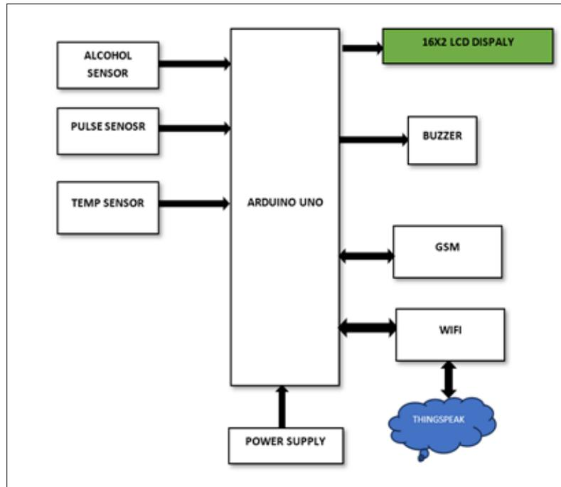
**Figure 1** Architecture for Liquor and Health monitoring system
