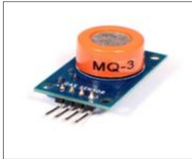
**Figure 3** Alcohol sensor (MQ-3)
