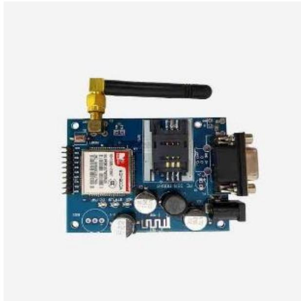
**Figure 8** GSM module
