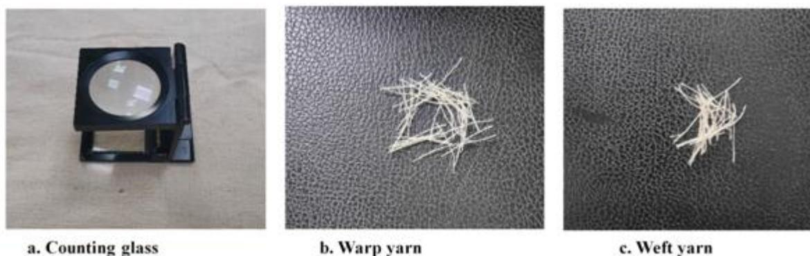
**Figure 1 a.** Depicts the method of EPI and PPI measurement using a magnifying glass. Figure 1 b. and 1c. shows the threads of wrap and weft yarn after removing from the fabric.
