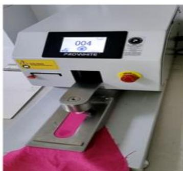
**Figure 7** The rubbing fastness test procedure
