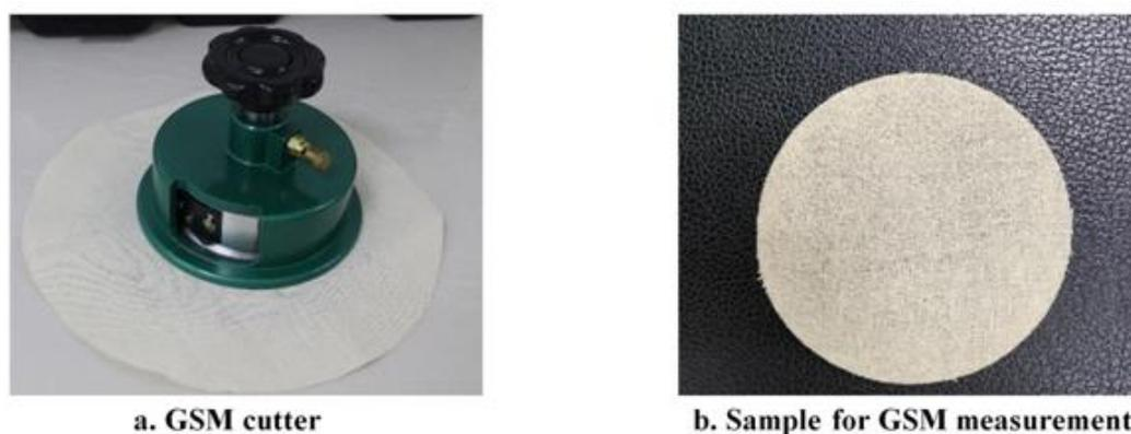
**Figure 2 a.** The process of fabric cutting using a GSM cutter has been shown, and in Figure 2 b. shows the cut grey fabric sample which was weighted in the electric balance.
