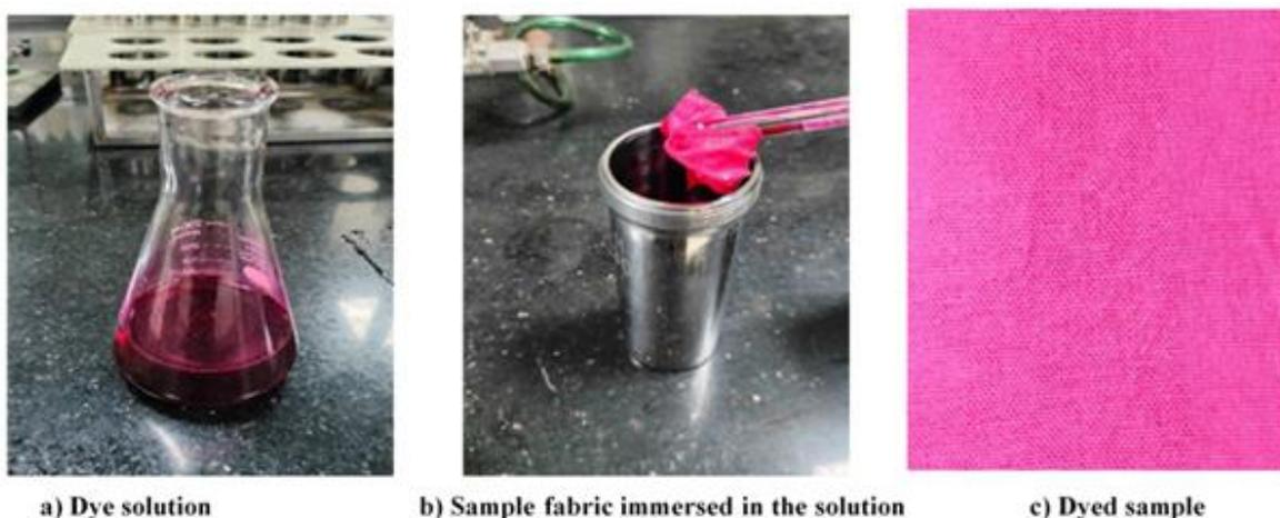
**Figure 3.** a) Depicted the preparation of dye solution. Figure 3. b) shows the sample fabric immersed in the solution and Figure 3. c) shows dyed fabric sample
