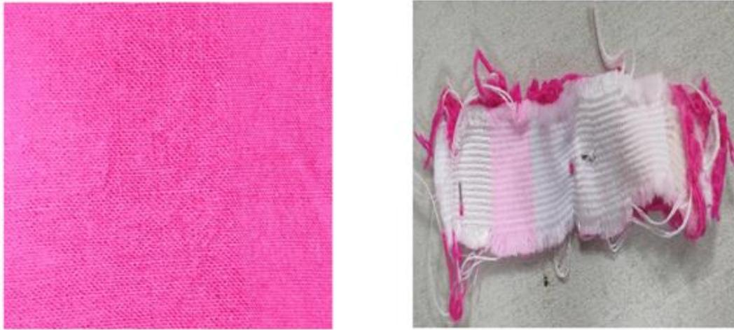
**Figure 8** The jute cotton blended dyed sample (left) and multifiber (right) after washing
