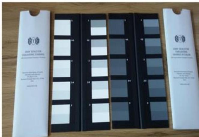
**Figure 6** The grey scale used for the grading
