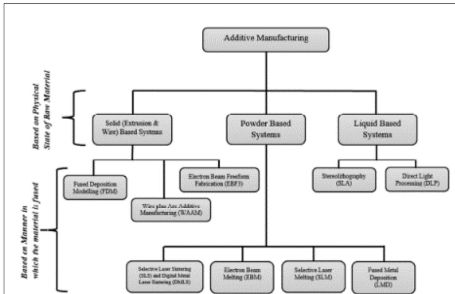
**Figure 1** Schematic of different types of 3D printing (Joshi, and Sheikh, 2015)
