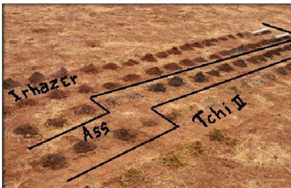
**Figure 6** Cuttings assemblage giving the lithostratigraphic succession of the study area.
