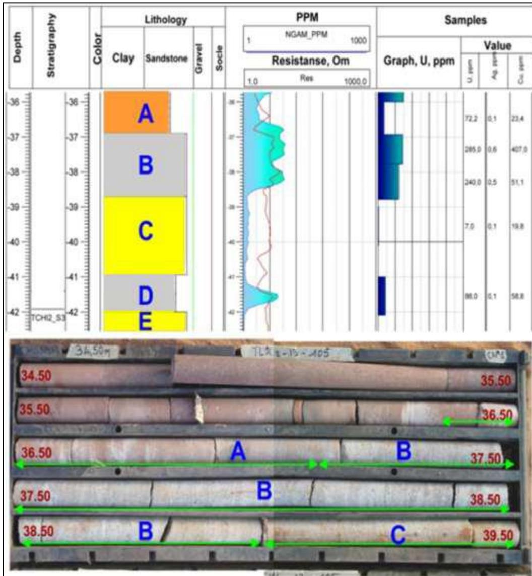
Figure 9 Correlation between lithology, logging and chemical analysis results.
