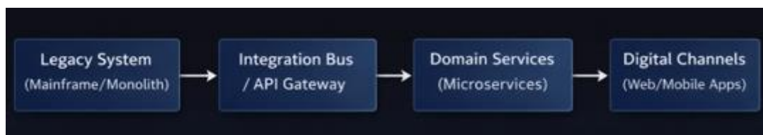
Figure 1 Incremental modernization architecture: legacy core systems coexist with new microservices via an integration layer, supporting modern digital channels
