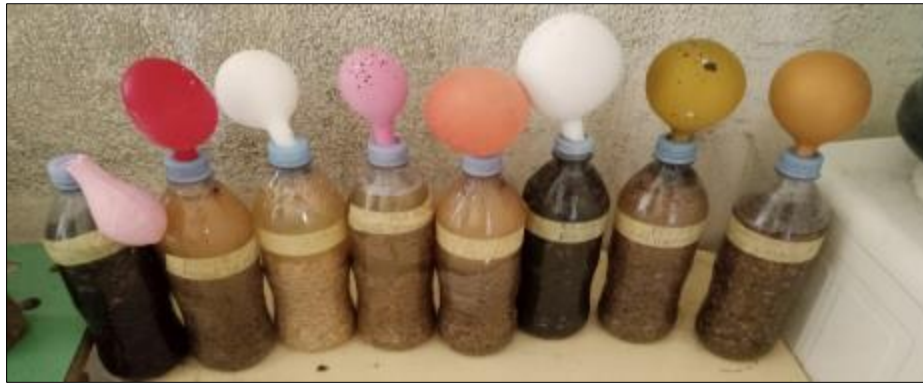
Figure 3 Implementation of the digesters at time T= During the experiment with agitation
