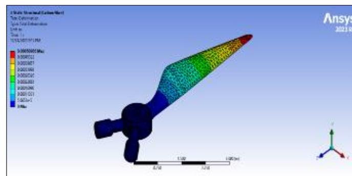
**Figure 4** Total Deformation; Carbon fibre
