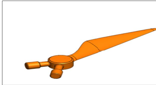
**Figure 9** Geometry of Blade Generated in Solidworks
