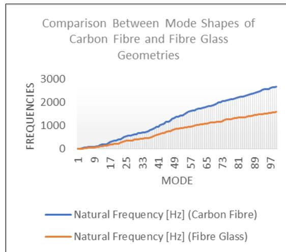
**Figure 8** Fundamental Frequency of Carbon fibre vs. Fibre Glass
