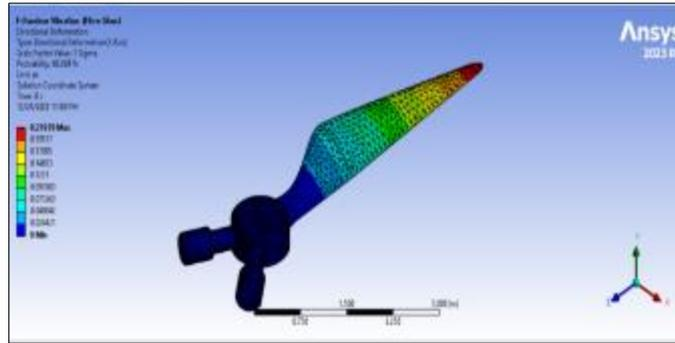
**Figure 5** Directional Deformation; Fibre glass
