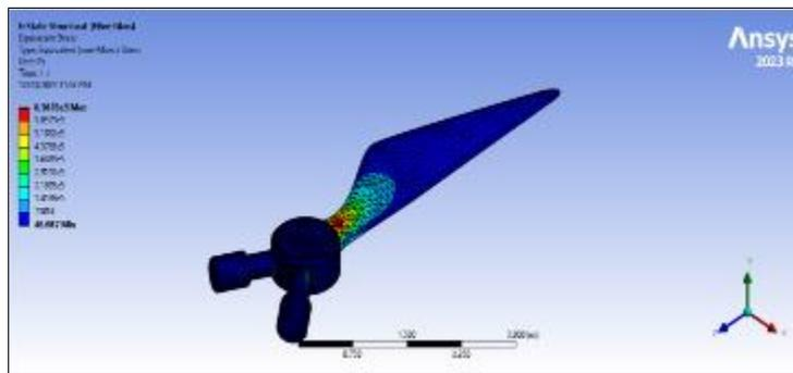
Figure 1 Equivalent stress; fibreglass
