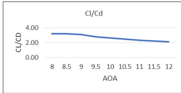
**Figure 18** CFD Simulation Result of Cl/Cd Against AOA
