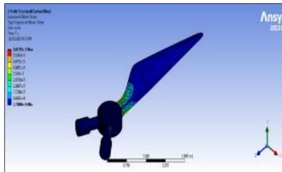
**Figure 7** Equivalent Elastic Strain; Carbon Fibre
