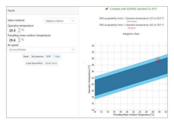
Figure 9 Analysis of classroom A<sub>EN</sub> with air velocity of 0.3m/s using CBE Thermal Comfort Tool.
