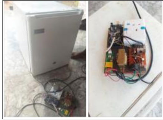
Figure 2 Physical set-up connection to acquire the measured data from the domestic refrigerator
