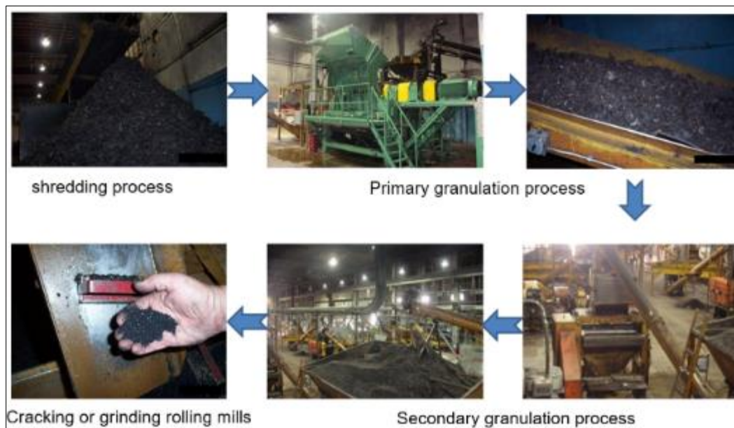
Figure 1 Process of producing crumb rubber
