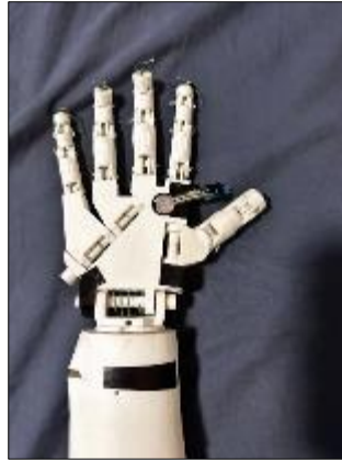
Figure 7 Prosthetic with an FSR mounted onto the upper palm
