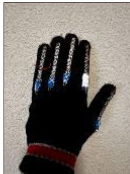
Figure 6 Glove with the flex sensors attached
