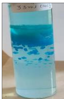
Figure 1 Crystal Growth of Copper tartrate in Silica gel
