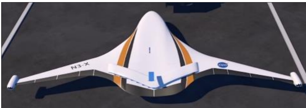
Figure 1 NASA conceptual design of BWB aircraft.[2]
