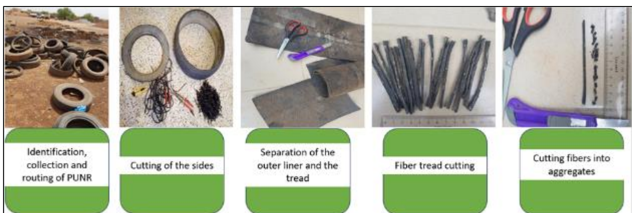
Figure 1 Synoptic diagram of the processing methodology to produce GPU from recycled tires
