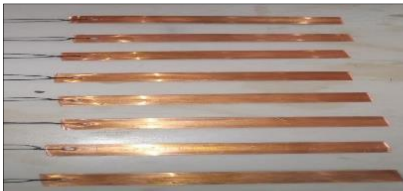
Figure 16 Metal coupons for corrosion test
