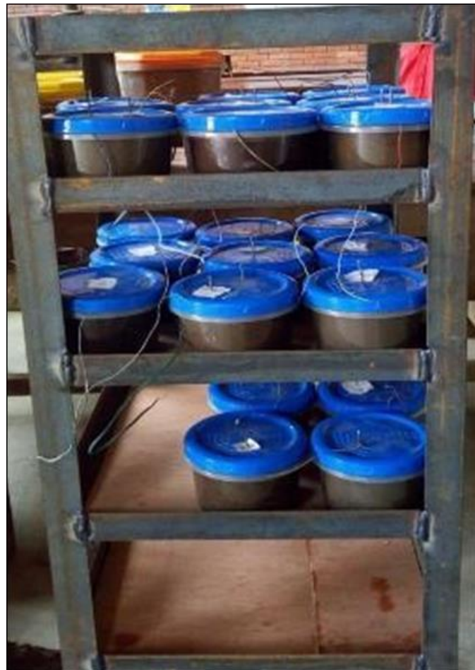
Figure 10 MFCs stacked and connected to power
