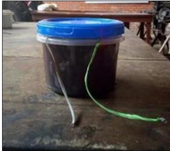
Figure 9 A prepared microbial fuel cell
