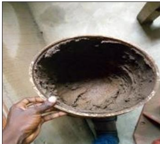
Figure 7 Prepared Slurry for the MFCs
