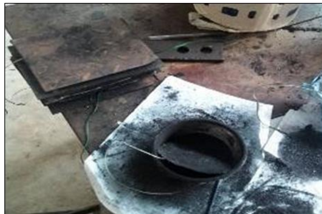
Figure 8 Preparation of Electrodes using Stainless steel mesh and Activated Carbon
