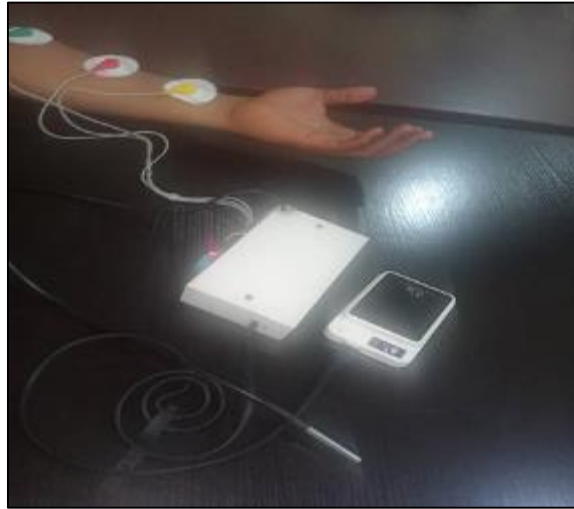
Figure 4 Wearable sensor nodes for ECG and Temperature during operation
