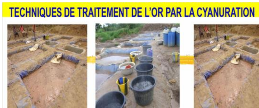
Figure 3 Cyanidation gold processing technique
