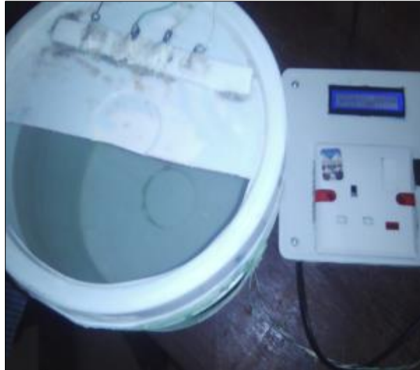
Figure 13 Permanent Construction of the Wireless Water Level Control System
