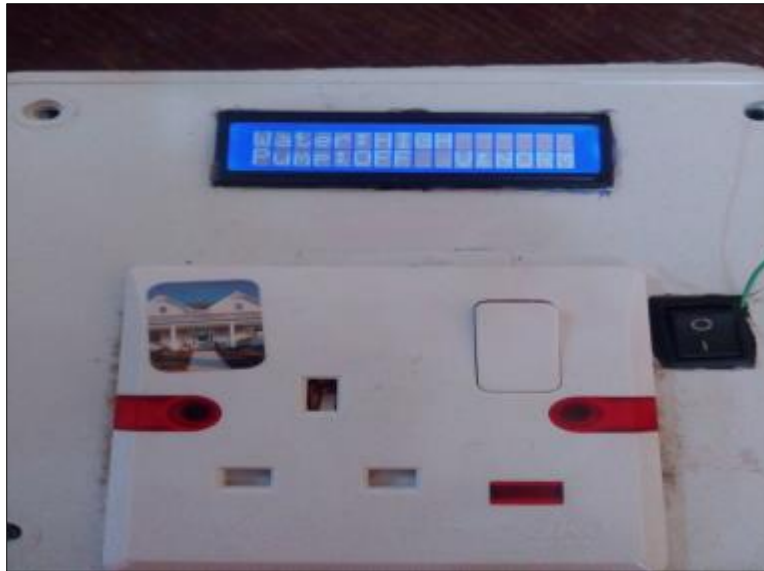
Figure 14 Testing of High Logic State of the Water Level Control System
