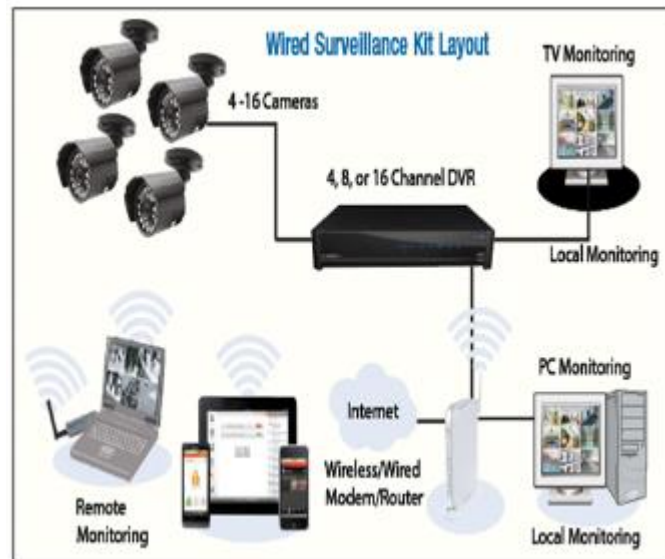
Figure 1 Physical network set-ups
