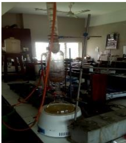
Figure 13 Extraction of fat from the seed using the Soxhlet apparatus
