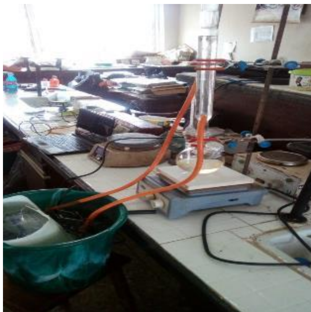
Figure 6 Batch trans-esterification reaction set-ups
