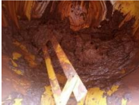
Figure 3 Sticking the mixture in the mixer with more than 20% water.
