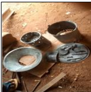
Figure 7 Assembling the various parts of the primary- and secondary-source cookstove
