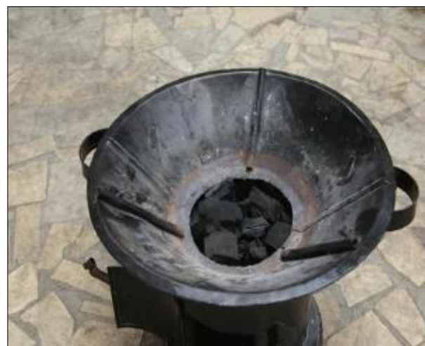
Figure 11: Hearth filled with coal
