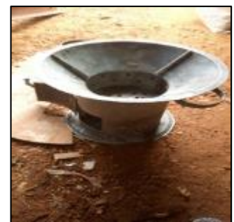
Figure 7 Assembling the various parts of the primary- and secondary-source cookstove
