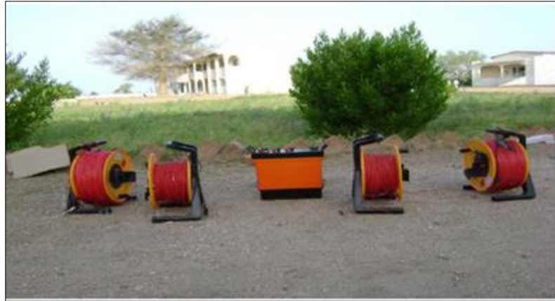
Figure 10 ABMN terrameter for measuring electrical prospecting
