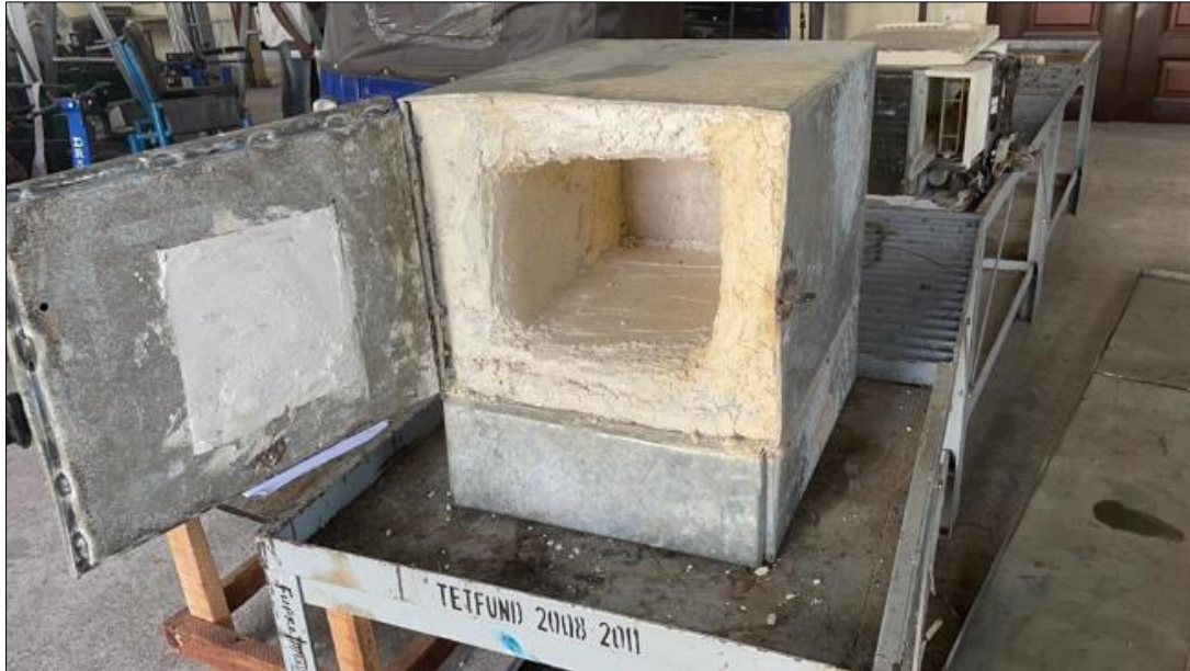
Figure 9 Fabricated electric heat treatment furnace
