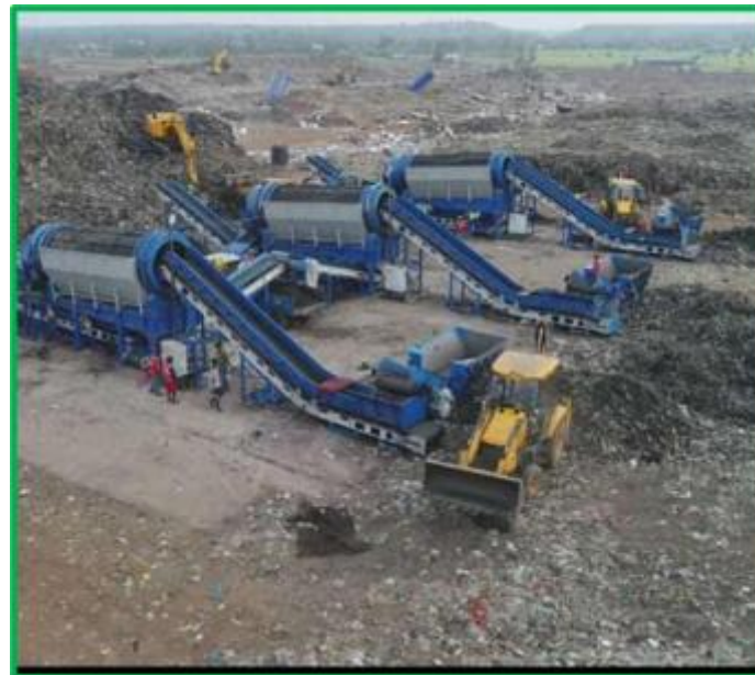
Figure 3 Trommelling machine segregating waste on landfill
