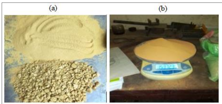
Figure 5 (a) pulverization of the soil, (b) weighing of the soil
