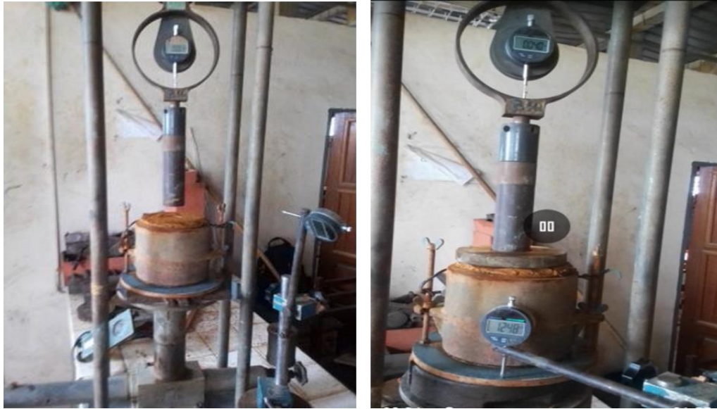
Figure 6 Penetration test for CBR
