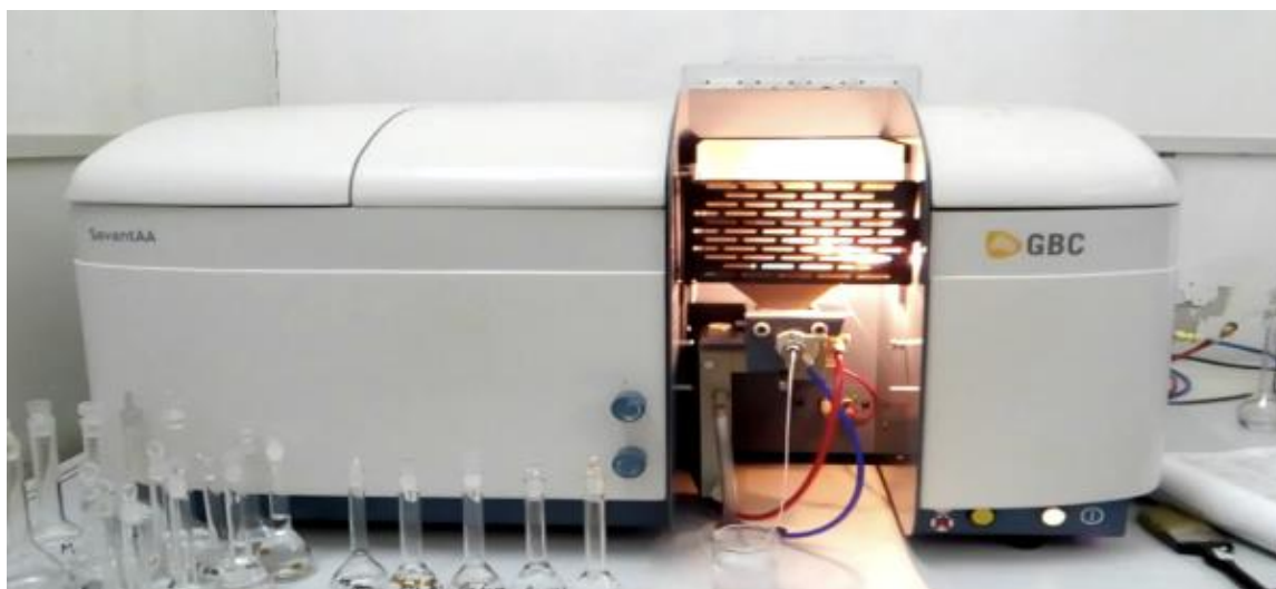
Figure 1 GBC 908PBMT Model Flame Atomic Absorption Spectrophotometer.
