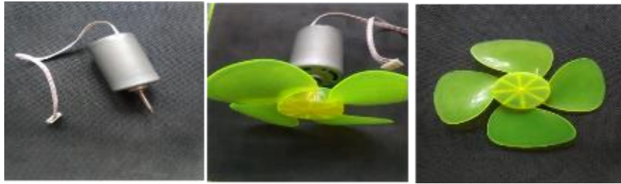
Figure 2 Parts of the wind generator
