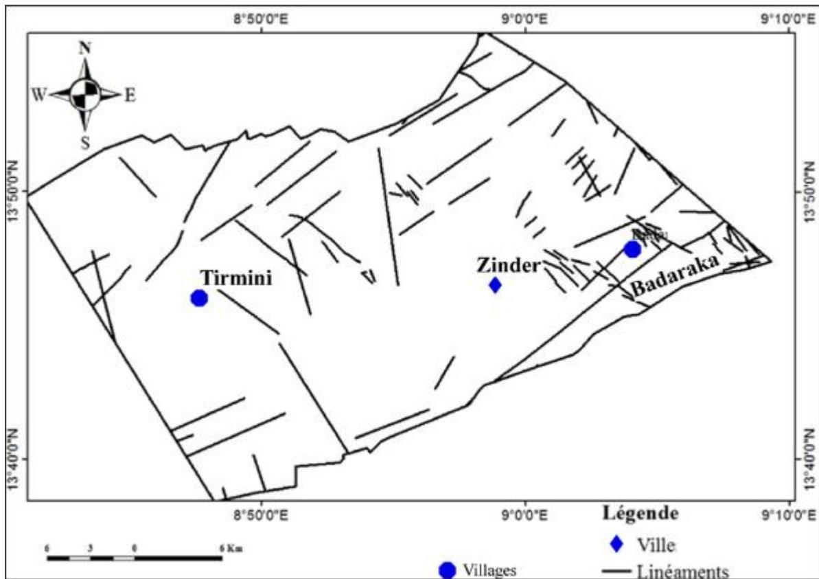
**Figure 3** Linear map deduced from Landsat 8 images and aeromagnetic images of the study area
