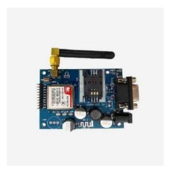
Figure 8 GSM module
