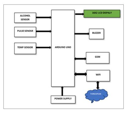
Figure 1 Architecture for Liquor and Health monitoring system
