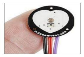
Figure 4 Pulse sensor
