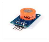
Figure 3 Alcohol sensor (MQ-3)
