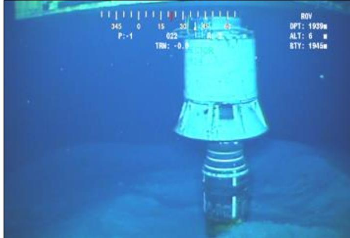
**Figure 16** Phase 2: Seating the BOP in the wellhead
