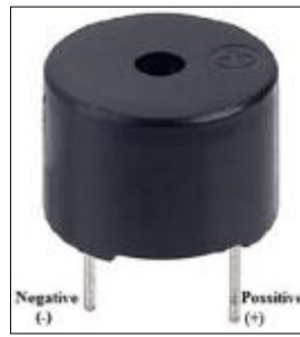
Figure 6 Buzzer used for early warning system
