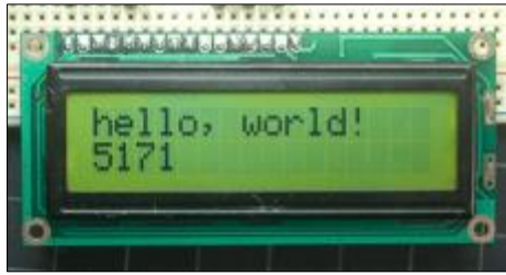
Figure 5 LCD Display for IoT-based flood monitoring early warning system
