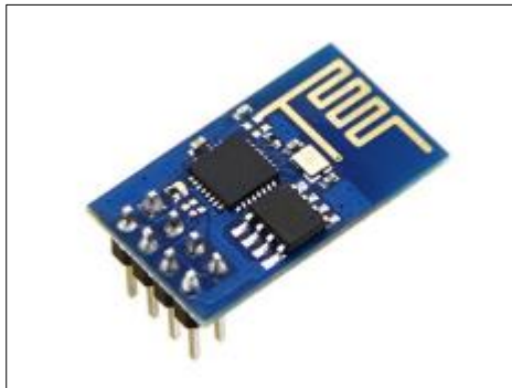
Figure 4 Wi-Fi module used in IoT-based flood monitoring system
