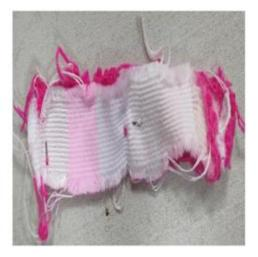
Figure 8 The jute cotton blended dyed sample (left) and multifiber (right) after washing
