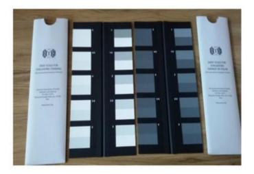
Figure 6 The grey scale used for the grading
