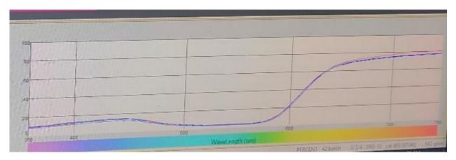
Figure 9 Reflectance curve of cotton and jute-cotton blended dyed fabric
