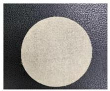
b. Sample for GSM measurement
