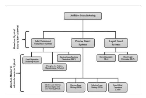
Figure 1 Schematic of different types of 3D printing (Joshi, and Sheikh, 2015)
