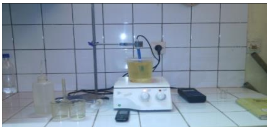
Figure 2 Photograph of the experimental montage of iron precipitation
